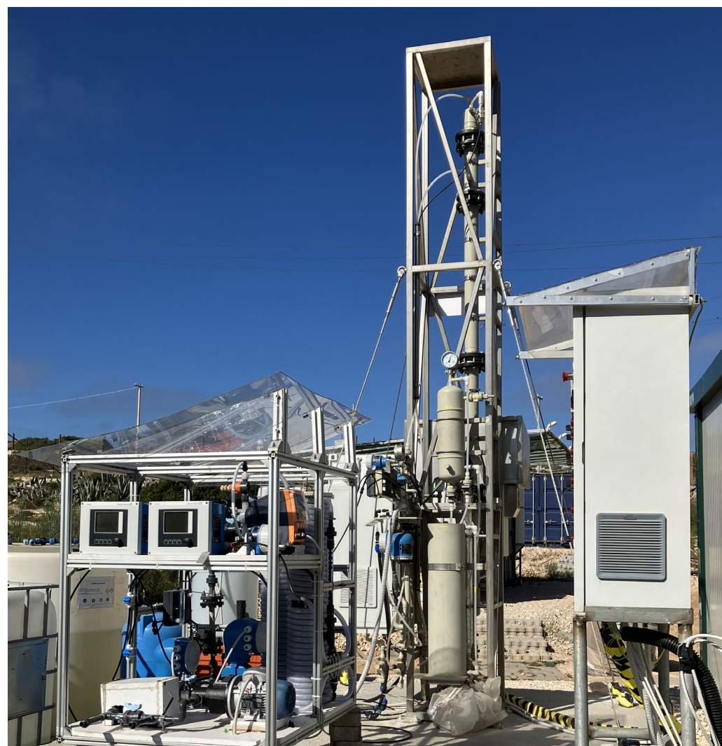
CO 2 extraction column + CO 2 injection skid
